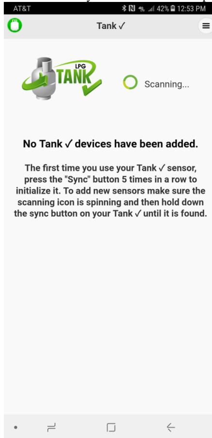
3. While the app is scanning, press the sensor SYNC button a minimum of 6X quickly. *Note: The first 5X awaken the sensor from sleep mode. It is only in sleep mode from the factory. Once awake, the sensor will never go into sleep mode again; and only 1 press is required to re-SYNC or connect to a new device.*
